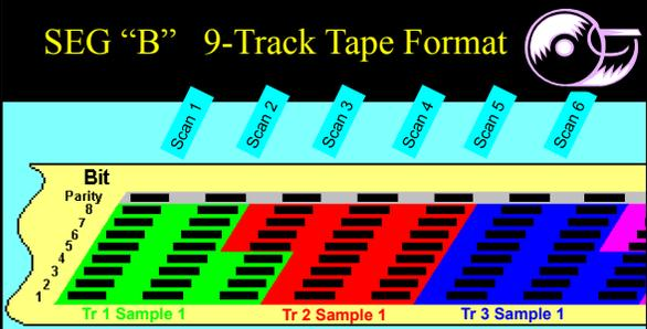
The diagram shows a 9-track tape with six scans. Each scan contains bit patterns for three samples (Tr 1 Sample 1, Tr 2 Sample 1, Tr 3 Sample 1). The bits are organized into a grid with 8 bits per track (Parity, 7, 6, 5, 4, 3, 2, 1).
