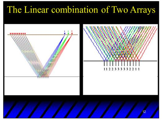
Consider a combination of a 9-element receiver array with an element spacing of  $\Delta X$  and a 3-hole shot array with and hole spacing of  $2 \Delta X$ . For 2-D programs the source array and receiver array will be in the same azimuth.
