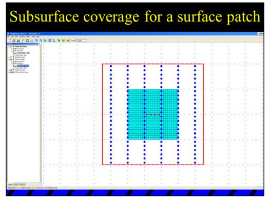
Here is a 3D survey with an active patch of 6 lines by 24 stations (only for teaching purposes). When one salvo of source points is completed near the center of the patch, what subsurface coverage is obtained?
