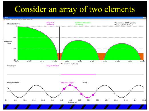
This is the response function for 6 geophones separated by 5 meters for an effective length of 30 meters. Again, notice that the effective length of the array coincides with the wavelength of the first notch in the response function. The second notch occurs when exactly two wavelengths exist across the array or at a wavenumber of
