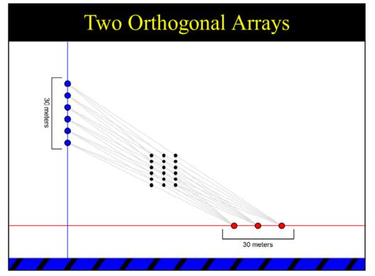
This diagram shows 6 geophones in-line along a north-south receiver line. The geophones are spaced 5 meters apart for an effective array length of 30 meters.
