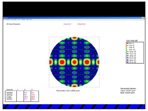
The 3-D array response function shows the theoretical attenuation in dB as a color, wavenumber as radial distance from the center of the plot to the edge of the plot (wavenumbers of 0 to  $0.2 \text{ m}^{-1}$  or wavelengths of  $\infty$  at the center down to 5 meters at the edge of the response. Source-receiver azimuth is represented by degrees of rotation around the plot.
