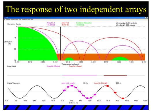
A 9-element geophone array with  $\Delta X=3.33333$  meters will have an effective length of 30 meters. Its response is shown above in the violet line curve.
