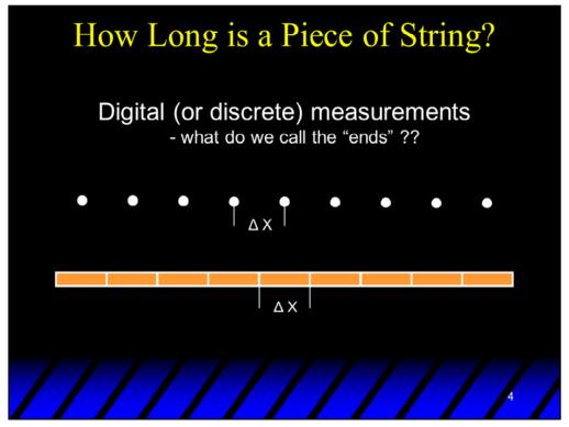
9 points separated by a distance of  $\Delta X$  will represent a distance from the first point to the last point of (9-1) x  $\Delta X$ . This is called the "Measured" length and is given as (N-1) x S where N is the number of elements and S is the separation between
